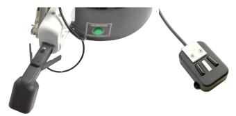
User buttons status are provided to the software interface. The end effector orientation can be modified.
