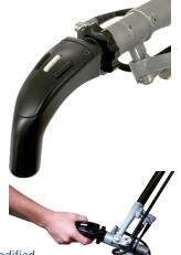
The end effector orientation can be modified. The device can be configured in up-side-down position.
